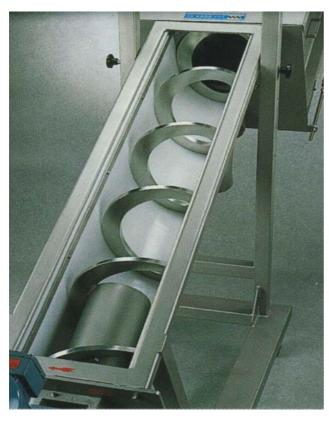
The spiral press is consisting of a U-trough made of folded plates. It is furnished with inlet hoppers of adequate size to suit the discharge chute of the screen.
