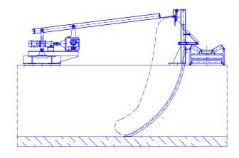
Screening discharge to drainage channel, belt conveyor or screw conveyor.
