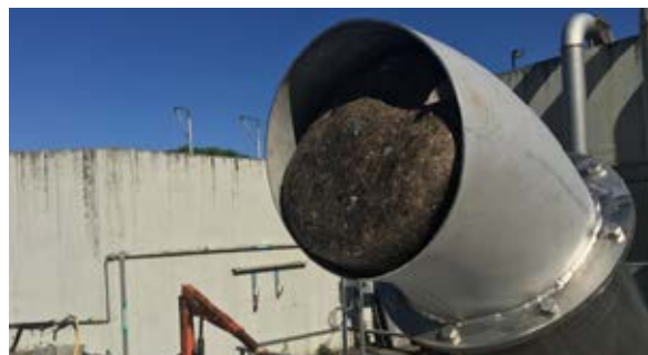
W-Co series screw wash compactor with the unique duck neck discharge pipe, build as horizontal screw for hopper loading and integrated washing section of screenings.
