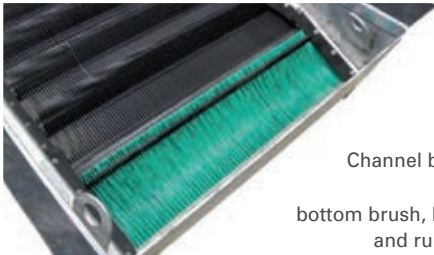
Rotary brush inside discharge hopper
