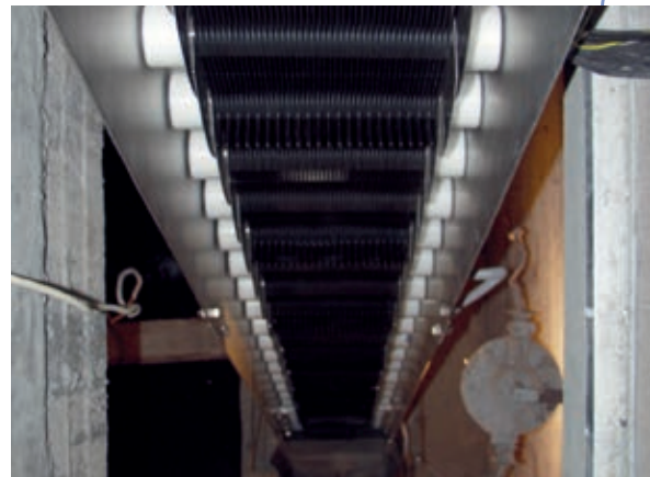
Endless step chain with hooks of high durable glass fibre reinforced plastic
