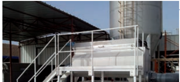
Application: Tertiary treatment, pre-filtration before Reverse Osmosis; size comparison of MSS B10-3000 in the front and the sand filter in the back, which has only one quarter of the MSS filter capacity.
