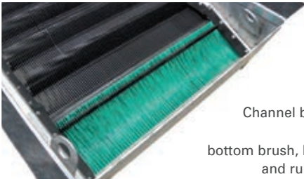
Rotary brush inside discharge hopper
